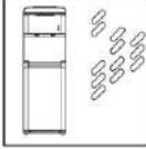
2. IT IS ALLOWED TO CONNECT THE DEVICE TO THE NETWORK ONLY AFTER FILLING ITS CONTAINERS WITH WATER. OPERATION OF THE DEVICE WITHOUT WATER IN CONTEINERS OR WITHOUT WATER IN A BOTTLE IS NOT ALLOWED.
